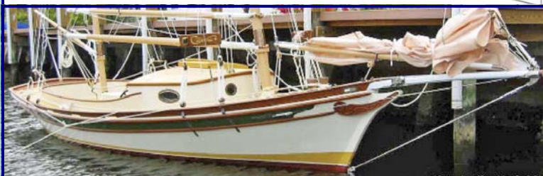
Czarina: a custom 27' centerboard solar/electric ketch designed for an experienced sailor in The Bahamas. Built by Covey Island Boatworks of wood/epoxy. Featured in the Sept/Oct. 2007 WoodenBoat magazine.
